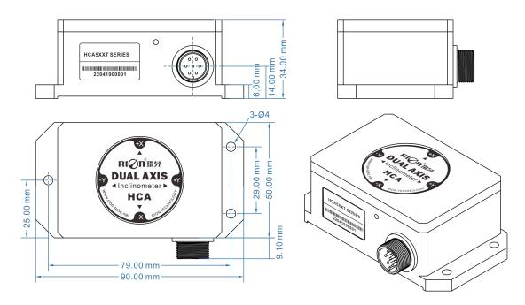
Shell size: L90×W59×H34mm Installation size: L79×W29×H6mm ounting screws: 3M4 screws
