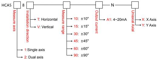
E.g:HCA518T-10-A1-N-X:Single / standard horizontal measurement/±10° measure range /4-20mA output /X Axis.
